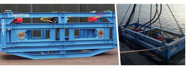
The TwinProp subsea excavation system is the next generation, state-of-the-art development of the widely proven controlled flow excavation technique. Counter-rotating propellers are used to produce two high volume columns to rapidly excavate the seabed.
