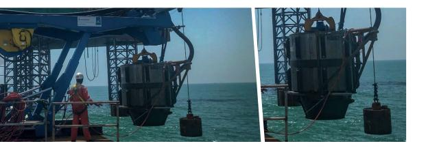
Deployed over a vessel side and operated remotely from its deck, the SP6000 works by producing a controllable column of water, the pressure of which effectively excavates the seabed.
