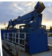
The National Crane comes complete with skid assembly suitable for deck mounting and a 22kW electric safe area HPU mounted on grillage. The fitted winch is capable of lifting 1te at max outreach.
