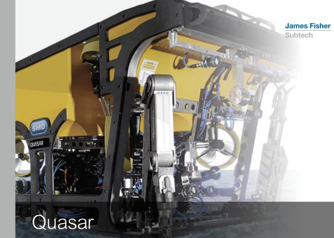
The high performance work class remotely operated vehicle (ROV) enables precision manipulative tasks even in high currents.
