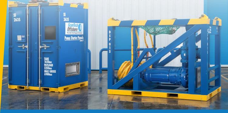
ScanTech is able to provide complete temporary fire pump back up, our standalone dual submersible pumps and topside booster pumps provide ample volume and flow rate should the rigs fire systems need to remain operational during the decommissioning process. Our systems can provide temporary cover during the deconstruction of the installation.
