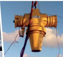
The T4000 excavation tool generates a large volume column of water which travels vertically down to the seabed at a velocity of up to 10m per second.
