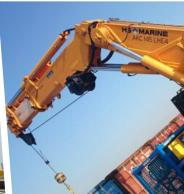
The AKC 145 LHE4 comes complete with a dedicatedHPU, transport base with incorporated seafastening plates. Benefiting from dual controllocal and Canbus remote control allows theoperation of the crane both from the dedicatedoperator's seat and also on deck ensuring bestline of sight at all times.
