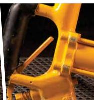
The Stanley CH 18 is a portable hydraulic chipping hammer, fully sealed for underwater use.
