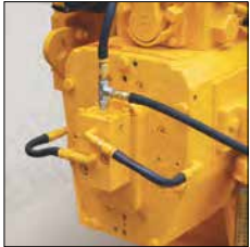
LS2000R with overload protection
