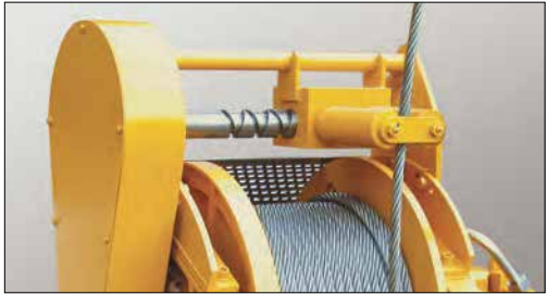
Spooling device on LS5000R
