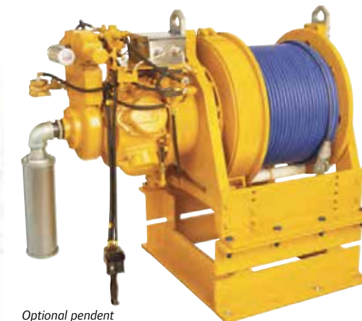
Optional pendent for secondary local control
