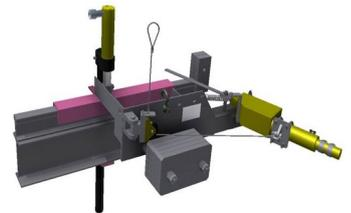
**The Column Cutter** was part of a suite of tools designed for the removal of steelwork from Bay 9, Pile Fuel Storage Pond at Sellafield. A hydraulic reciprocating saw was mounted to a bespoke bracket, with integrated clamping system. This allowed the assembly to be deployed onto the columns of the shield plug support frame, and then clamped in place. Using a pulley system, the blade of the reciprocating saw was then driven through the column, separating the upper steelwork from the lower.
