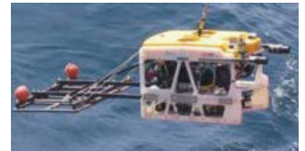
Survey skid with TSS pipe tracker
