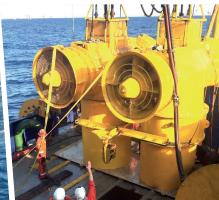
The Twin T8000 excavation tool generates two large volume columns of water which travel vertically down to the seabed at a velocity of up to 10m per second.
