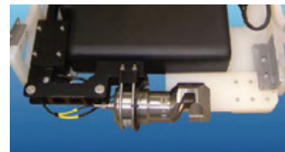
Cable cutter skid
