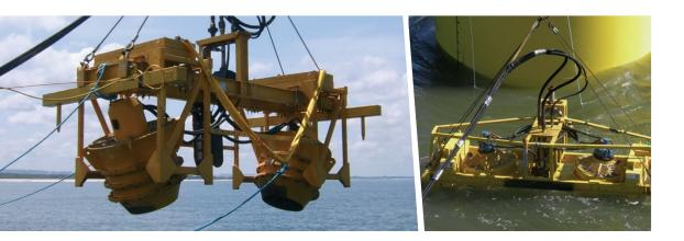
The Twin R2000 subsea excavation tool generates two controllable columns of seawater which travel vertically down towards the seabed at a velocity of up to 10m per second.
