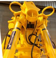
Fisher Offshore's orange peel grab can be quickly and efficiently operated via deck controls/diver control stand or ROV hot stab set up.
