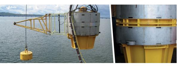
Deployed over a vessel side and operated remotely from its deck, the SP12000 works by producing a controllable column of water, the pressure of which effectively excavates the seabed.
