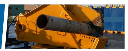
The 2835Te Hydraulic Shear is a versatile tool capable of performing fast and efficient scrapcuts on a variety of different grade materials of varying size and thickness.
