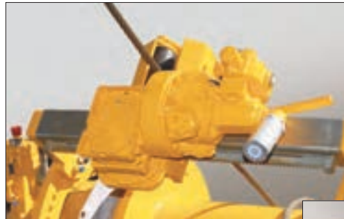
2 hp radial piston drive motor. Fully enclosed oil bath gear box
