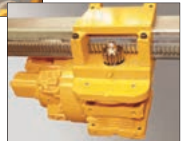
Precision cut rack & pinion drive assembly
