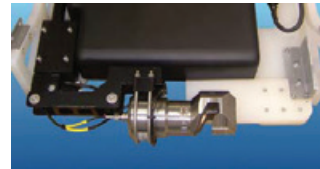
Cable cutter skid
