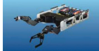
Manipulator skid with grabber arm
