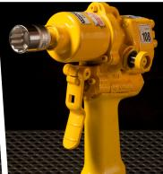
The 1/2" square drive impact wrench delivers torque up to 500 ft lbs and can tighten and loosen nuts and bolts and drive lag screws. Trigger guard and hi-visibility yellow paint is standard.
