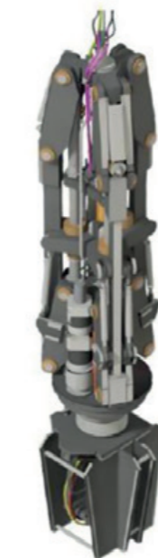
JFO's abrasive water jet internal cutting head
