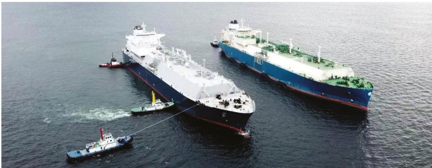
JF Fendercare conducted break-bulk LNG STS operations for a leading energy company, transferring cargoes of varying quantities. Requiring meticulous planning and preparation, this allowed the cargo to be split from a large vessel to numerous smaller vessels to overcome local terminal restrictions.
