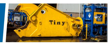
The 1950Te Hydraulic Shear is a versatile tool capable of performing fast and efficient scrap cuts on a variety of different grade materials of varying size and thickness.
