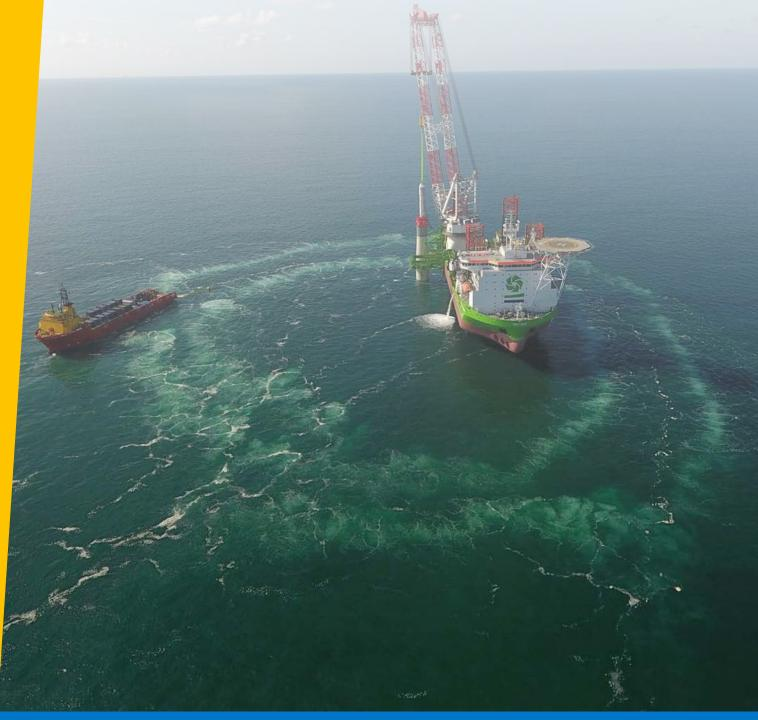
ScanTech Offshore support offshore wind farm construction in Europe, UK, Asia and the US with a focus on environment protection. ScanTech support Big Bubble Curtain (BBC) Operations with the supply of Oil Free (Class 0) compressed air delivery packages.
