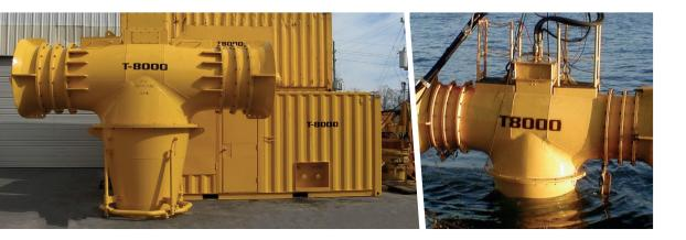
The T8000 excavation tool generates a large volume column of water which travels vertically down to the seabed at a velocity of up to 10m per second.
