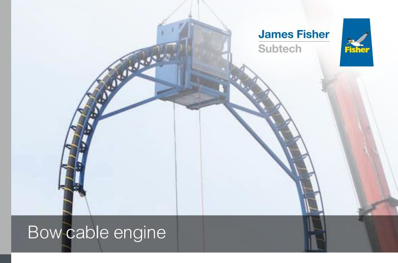
The Smartquadrant – E bow cable engine has been designed to assist in loading various cable types from fibre optic to medium sized power cables. The complete system consists of two quadrants and one central electrically-driven hydraulic power unit with a wired remote control. As the system is electrically-driven, it can be used both for loading cables in harbours and for transpooling cables on-board cable lay vessels or freighters.
