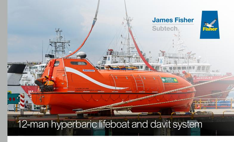
The self propelled hyperbaric lifeboat (SPHL) is an enclosed motor propelled survival craft equipped for the evacuation of 12 divers under pressure, fully compliant with IMO requirements. Provision is also made for 72 hours life support for the divers while awaiting rescue.
