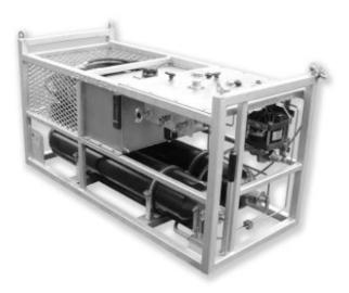
The Accumulator pump is a portable unit designed for the hydraulic opening and closing of hydraulic cutting equipment. This is especially advantageous in emergency situations where the cutter is required to operate with a fast reaction time.
