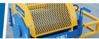
The BFG10 is a single drum hydraulic powered winch driven by a single speed axial piston motor via a planetary reduction gearbox. Where required this winch can be adapted for subsea deployment including ROV operation.
