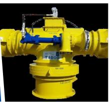
The T4000A excavation tool generates a large volume column of water which travels vertically down to the seabed at a velocity of up to 10m per second. In addition, a high velocity jet of water, located in the centre of the mass flow column facilitates the cutting of hard soils.
