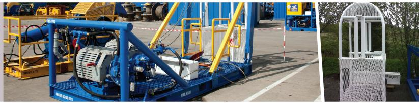
Fisher Offshore's Diver LARS is a hydraulic A-Frame with diving cage, specifically designed to provide a robust operating design to limit the amount of deck space needed.
