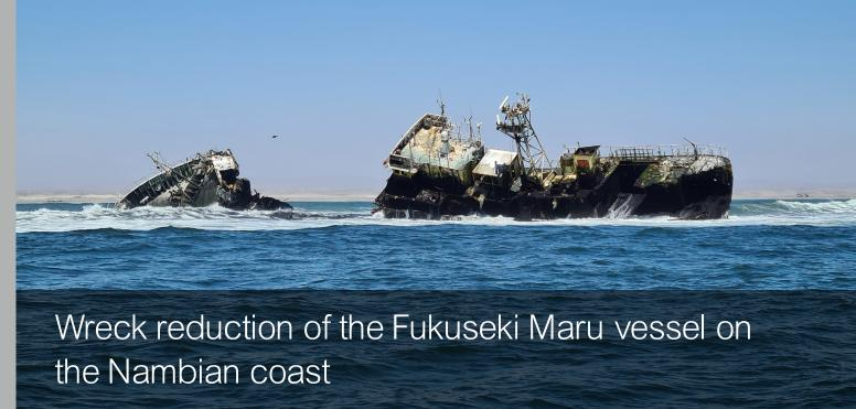
James Fisher Subtech (JF Subtech) successfully reduced the size of the Fukuseki Maru vessel wreck claimed by the treacherous waters along the coast of Namibia. The trained team blasted the vessel to weaken the integrity of the structure which allowed sea conditions to speed up the breakdown process of the structure.
